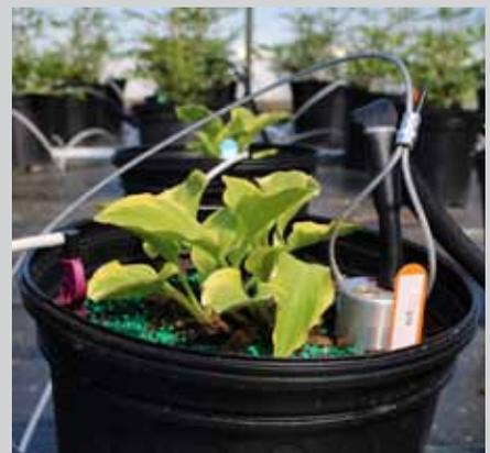
Tensiometer probe monitoring soil moisture.
